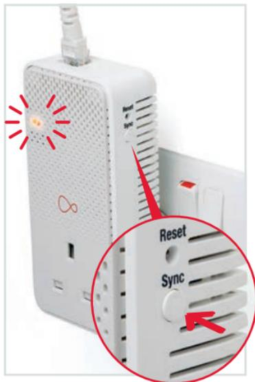
Within **2 minutes** press the Sync button on the second Booster for **3 seconds**. The connection light will also flash rapidly.
